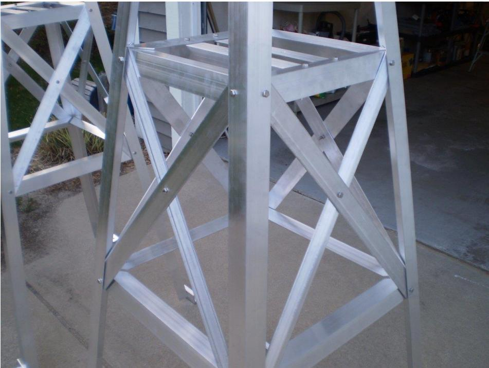
7. Attach the 2 rotor shelves to 2 of the upper shelf brackets with 4 each  $\frac{1}{4}$ "-20 x 1" bolts, lock-washers and nuts as shown below. Verify that all rotor mounting holes are 3.31" (Yaesu) or 3.0" (Hy-Gain) or 2.5" (MC-10) apart, then tighten these bolts securely.
