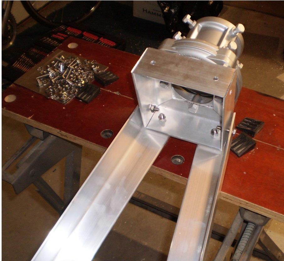
5. Assemble a second leg assembly identical to the one assembled in Step 3. Lay this assembly on top of the first leg assembly. The feet attachment holes should be facing up. Attach to the top assembly as shown below. Use 4 each  $\frac{1}{4}$ "-20 x 3/4" bolts, lock-washers and nuts. Hand-tighten the hardware at this time.
