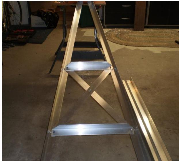
4. Attach the leg assembly to the top angle bracket assembly as shown below using 4 each of the 1/4"-20 x 3/4" bolts, lock-washers and nuts. Hand-tighten the hardware at this time.
