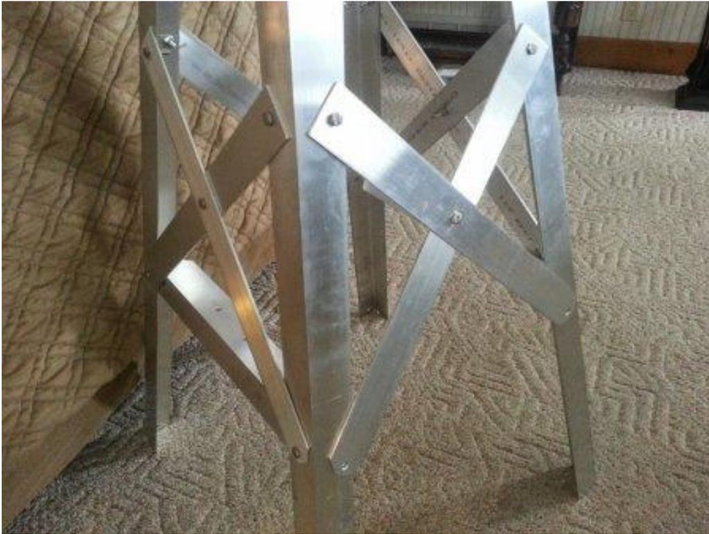
8. Attach the 2 remaining lower shelves to the tower assembly, using  $\frac{1}{4}$ "-20 x 1" bolts, lock-washers and nuts. Place each bolt through the X-brace and leg with just a couple threads showing on the other side. Place the lower shelf carefully on each bolt, then secure with a lock-washer and nut. When both shelves have been installed, tighten all hardware securely with a wrench. See the image at left below.
